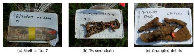
Figure 3.30: a) Unexploded shell from Cell No. 7 and (b,c) the two false alarms obtained by the SVM classifier using k and as discriminators.
