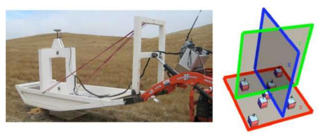
Figure 3.1: The MetalMapper during SLO site deployment (left) and its schematic diagram (right).
