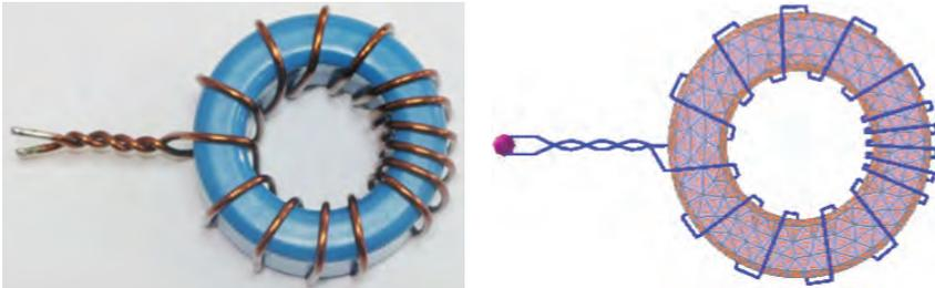
Fig. 105. Measured sample and model of coil
